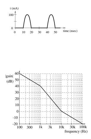
d) \*\*Note\*\* This part is not for the same PLL as parts a), b), c). For a PLL which uses as loop filter an integrator with phase-lead correction, with a natural frequency of 1 kHz, damping constant of 0.707, and an exclusive-or gate phase detector, estimate the maximum frequency step which can be applied to the loop without losing lock during this step. Also, estimate the settling time during such a transient.
