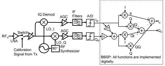
The radio must be able to handle signals from -80 to -30dBm with an SNR of 15dB. The A/D should have a 1V input signal. Received signals in the band of 2GHz with a bandwidth of 5MHz. The IF is at 10MHz. Fill in the following table so that the radio will operate properly:
