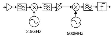
You must design the components of the radio to deliver a signal to the base band with a SNR of at least 10dB. In order to do this fill in the following table at a minimum:
