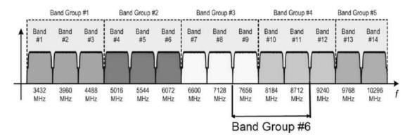
Design a LO network that takes a signal at 16896MHz and with SSB mixers, MUXs, and dividers generates all these frequencies.
