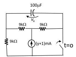
6) Analyze the circuit shown below and find the current in the capacitor  $I_c$ . The value X is the last digit of your student number. If your student number ends in 0 use X = 10. Note that the current source is sinusoidally varying. Note impedances are labeled on the diagram.
