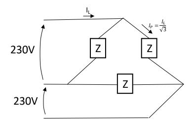
Power  $P = 3P_{\phi}$ =  $3 \cdot V \cdot I \cdot PF$ =  $3 \cdot V_L \cdot \frac{I_L}{\sqrt{3}} \cdot PF$ So  $2000W = I_L \cdot \sqrt{3} \cdot 230 \cdot 0.9$   $I_L = 5.58A_{rms}$  so  $I_{\phi} = \frac{I_L}{\sqrt{3}} = 3.22A_{rms}$ Then  $Z = \frac{V}{I} = \frac{|V|}{|I|} \angle (\theta_v - \theta_i) = \frac{230}{3.22} \angle \cos^{-1} 0.9 = 71.4 \angle 25.8\Omega$
