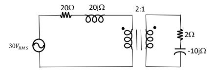
We first transform the impedance on the secondary to its equivalent resistance on the primary:
