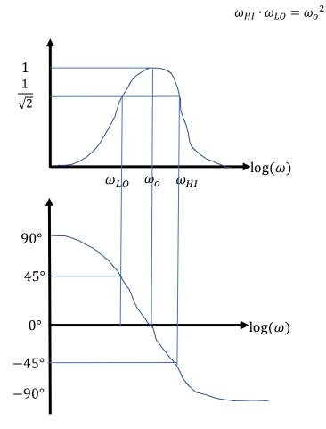
So small R = high Q = narrow bandwidth = high selectivity e.g. tuning or filtering. Now consider energy storage in the resonant circuit.
