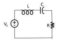
Find R,L, C to give a BP filter with  $\omega_o = 1000 rad/s$  , BW = 100rad/s (usually in Hz)
