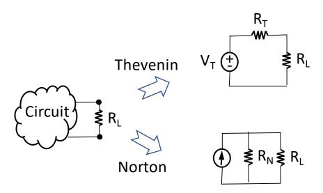
In both cases the current-voltage relation at the load stays the same. We can change the load value and the equivalent will accurately model the actual circuit!
