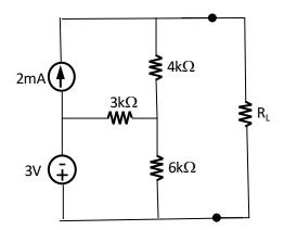
We start by removing  $R_L$  and finding the Thevenin equivalent. Note we only need  $R_{TH}$  to find  $R_L$  and we don't need  $V_{OC}$  unless we want to know the VALUE of the power transferred to the load.
