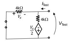
We note that  $V_x = -V_{TEST}$
