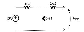
VTH = VOC =  $12V \times \frac{6k}{6k+3k} = 8V$  (note this is a simple voltage divider between the 3k and 6k resistor... why?? We assume open circuit at the terminals so no current flow through the 2k resistor thus it doesn't appear in the equation).
