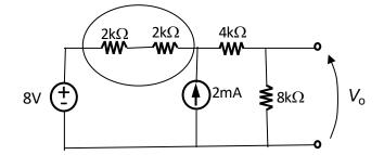
Which means the two circled resistors can be easily combined:
