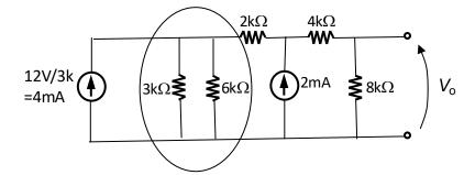
This puts two resistors directly in parallel for easy combining:
