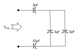
We note the two parallel caps have an overall capacitance of  $2\mu F + 2\mu F = 4\mu F$ .
