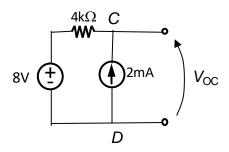
The new  $V_{TH} = 8V + 2mA X 4k = 16V$
