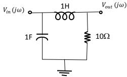
20) Derive the gain as a function of frequency:
