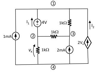
Write a set of equations sufficient to find all voltages and currents in the circuit.
